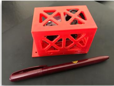
S4Arduino and S4Pi share the 1.5p PocketQube package. It is a 3D printed 5x5x7.5 cm plastic enclosure designed to hold the core processor, baseline sensors, battery, antennas, and additional sensors. About half the volume of the S4Arduino is available for optional sensors.
